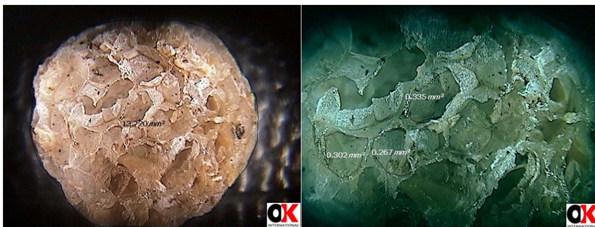
Figure 5. Microscope image ( \times 35 ) of the exemplary cross section profiles of the foam. [Color figure can be viewed in the online issue, which is available at wileyonlinelibrary.com .]
